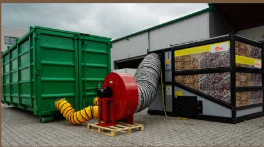
Container drying - also equipped with gill plate and heated with a Landritherm LA 250 woodchip furnace.
